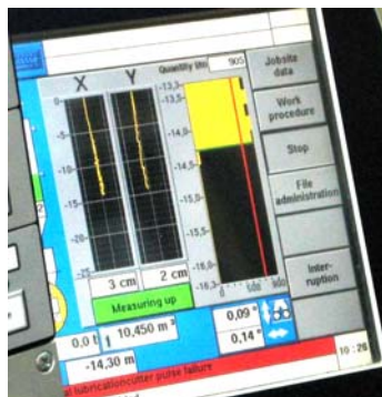
Figure 6. Guidance Control Panel
