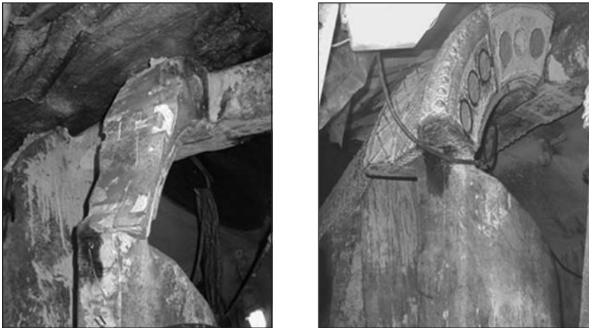
Figure 3. A bucket tool before repair showing wear through fixing bolts (left) and after repair (right)
