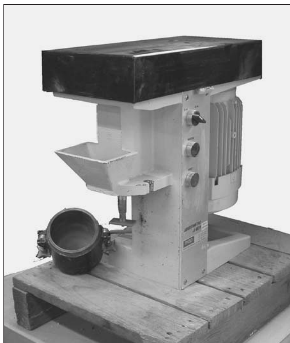
Figure 5. The LCPC abrasimeter test apparatus
