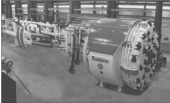
Figure 5. Robbins 261 TBM at their Solon, Ohio, facility
