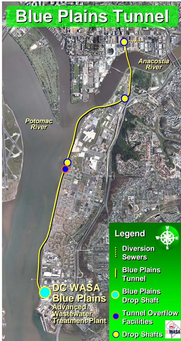
Figure 3. Blue Plains Tunnel Alignment
