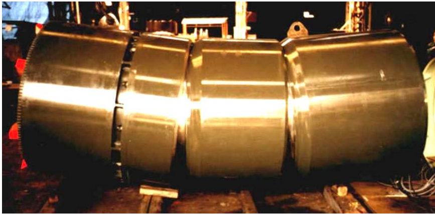
Figure 9. Double articulated Iseki TCT 1200 (57.9 in. [1,471 mm] OD)
