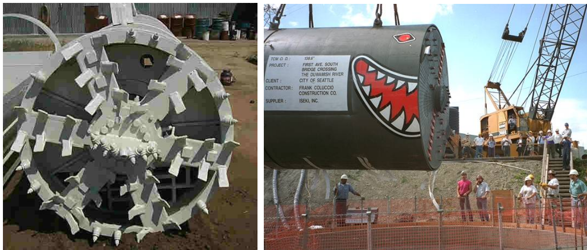
Figure 6. Examples of lightweight cutter wheels. Simple open-style cutter wheel design to allow the machine to be pushed forward and compact the loose soils with minimum rotation (left). Iseki MEPCB with the face completely closed and in a neutral position to provide breasting and compaction (right).
