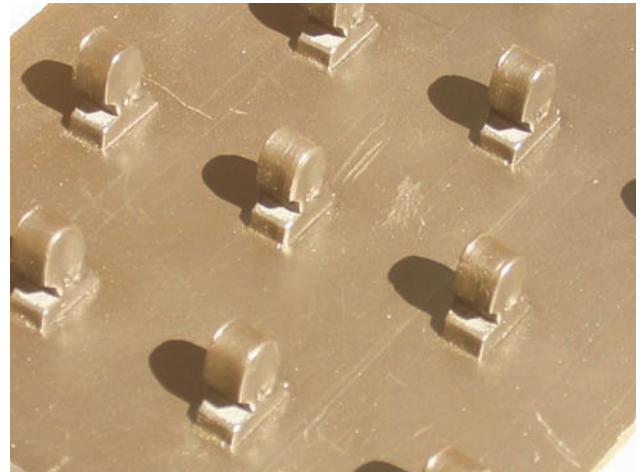
FIG 2 - Sample of high-density polyethylene (HDPE) with mechanical anchors.
